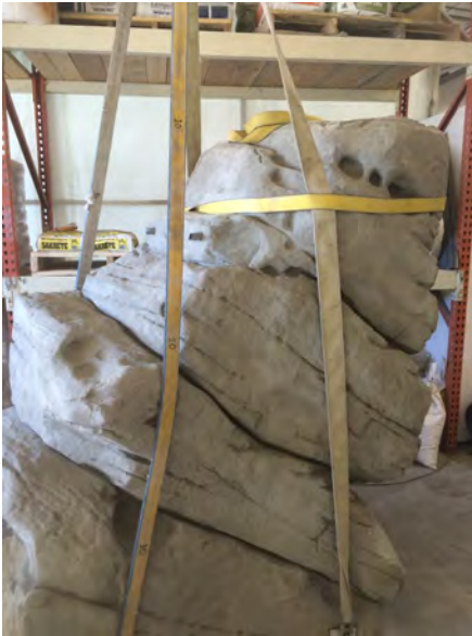
Example of ratchet strap choke on typical boulder. Strap is used to equalize load when lifting. (Note: this is not a Via Ferrata Boulder)
